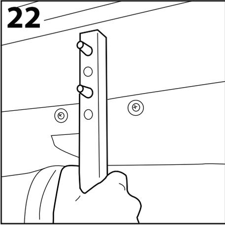
Replace the wheel support bar over the bolts using the alternative holes to make the adjustment of the door height.
