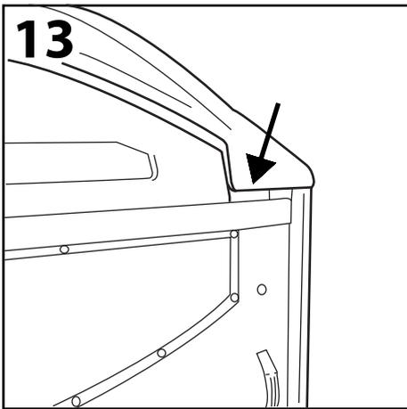
If the door is not level and there is a large gap between the hood, as seen above, the door wheel can be adjusted.
