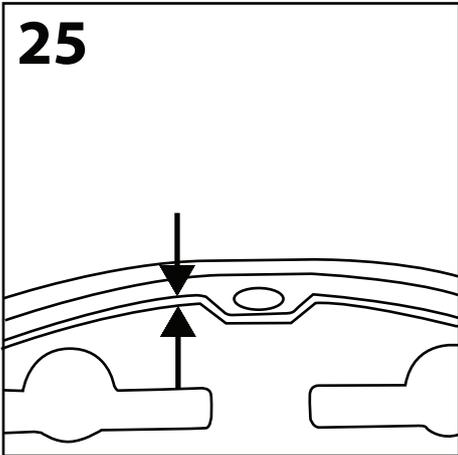
Ensure that there is an even gap around the perimeter of the door for optimum performance.
