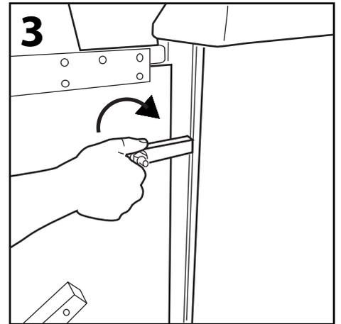
**3** To ensure that the door remains open whilst removing the wheeled bin, turn the door stay catch clockwise so that it is positioned horizontally.
