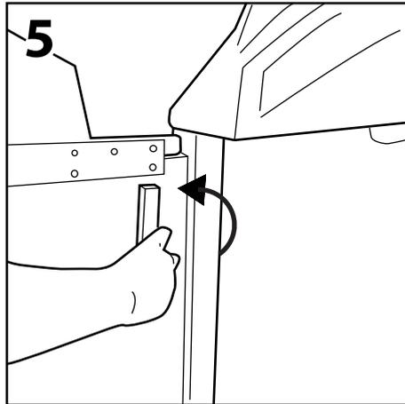
**5** After replacing the wheeled bin, remove the door stay catch by pushing upwards anticlockwise so that it is positioned vertically.
