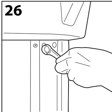
Using 17mm spanner, tighten the bolt at the top of each extrusion on the inside of the housing.
