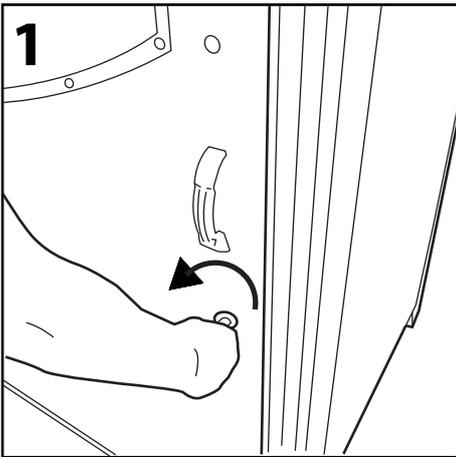
**1** Insert Glasdon Key into lock and turn anticlockwise to unlock the door. (Alternatively: Turn twist lock anticlockwise to unlock door.)
