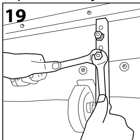
Using 17mm spanner, hold the nut closest to the wheel support bar. Using a second spanner unscrew the outermost nut and remove. Repeat on other wheel support bar fixing point.
