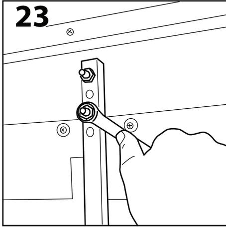
Making sure that the wheel support bar is 90 degrees to the door, replace the washer and first nut onto the bolt and tighten (do NOT overtighten).
