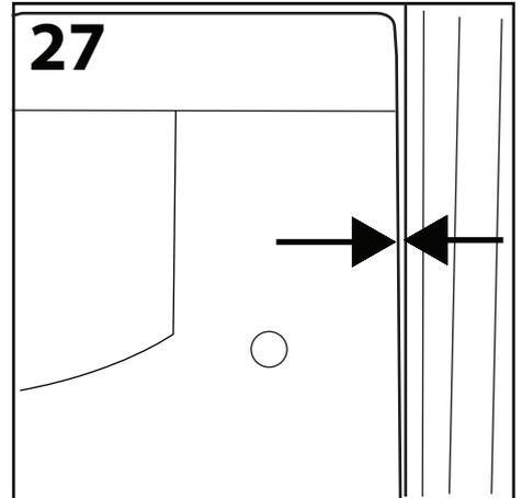
Close the door. Should the gap between the door and the extrusion be too small (as above) and the lock cover is catching, further tighten extrusion bolts (Fig 26). This will increase the gap.
