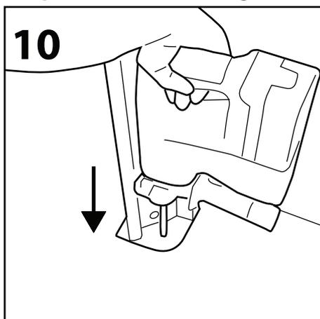
Using a 10mm masonry drill bit, drill through the hole in the spigot leg down into the concrete approximately 150mm deep.
