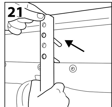
Lift the wheel support bar off the bolts, ensuring that the door is still supported.
