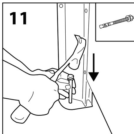
The fixing bolts (R) MUST appear as above with the nut and washer at the top of the bolt. Using a hammer, tap fixing bolt through the hole in the spigot leg until it is flush with the spigot plate.
