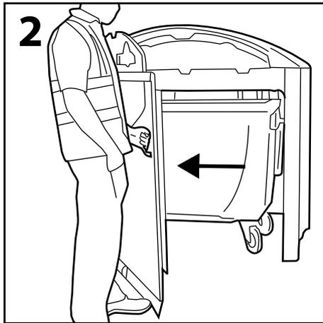
**2** Using handle pull door open to 90 degree position.
