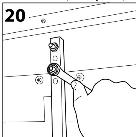
Using 17mm spanner remove the second nut and washer. Repeat on other wheel support bar fixing point.
