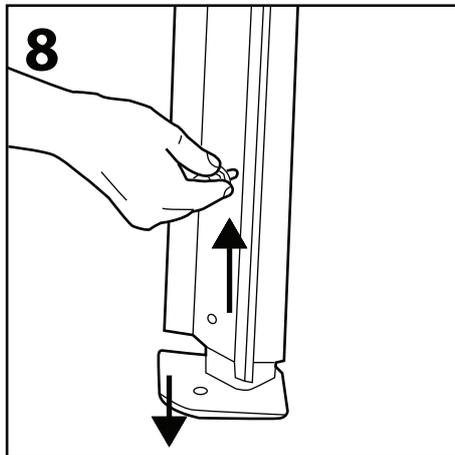
Lift the extrusion upwards and pull the spigot leg down to a more appropriate height ensuring that the housing is now level.
