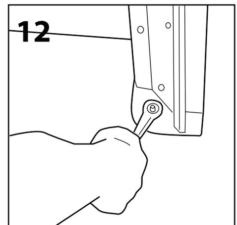
Tighten bolt using 17mm spanner. Repeat Figs 10-12 to ground fix the other three extrusions.
