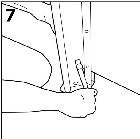
Using a 13mm spanner/socket unscrew the two bolts with washers on the inside at the bottom of the extrusions and remove.
