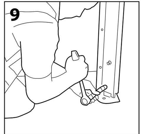
Replace the bolts and washers into the new holes within the spigot leg and tighten with spanner/socket. Repeat Figs 7-9 on the other legs that need adjusting.
