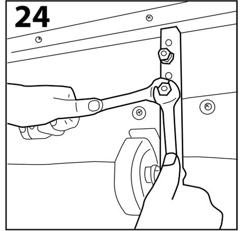
Holding the nut with the 17mm spanner, place the second nut over the bolt and tighten securely with a second spanner. Repeat Figs 23 and 24 using other fixings.
