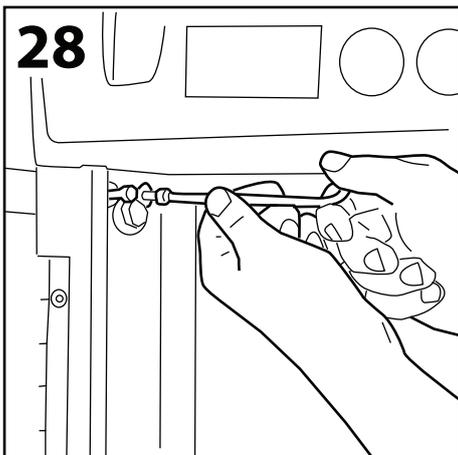
To reduce the gap between the door and the extrusion (opposite to Figs 26 and 27) on the inside at the top of the 4 off extrusions, tighten the 2 off screws with a 5mm allen key.
