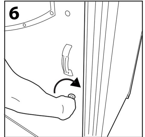
**6** Close the door and insert key into lock. Turn key clockwise to lock door. (Alternatively: Turn twist lock clockwise to lock door.)
