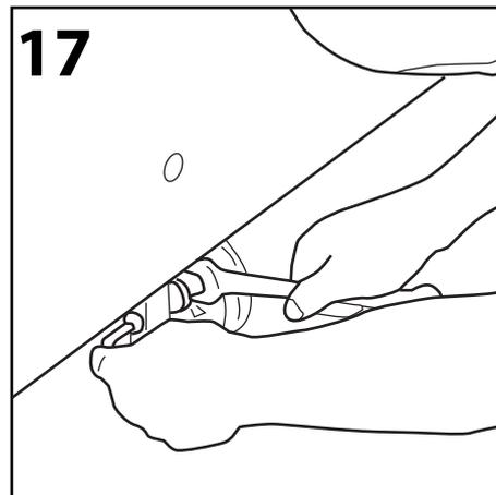
Once in correct position, tighten up nut (left of wheel) to lock the axle in place.
