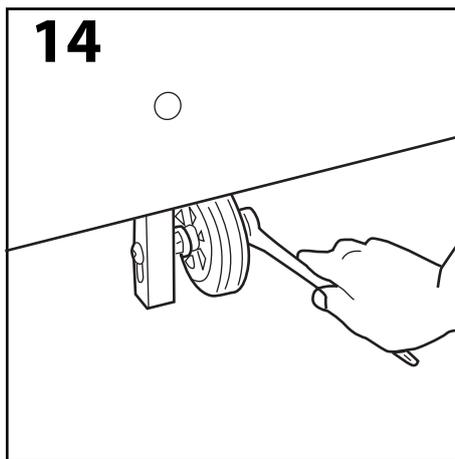
Using 17mm spanner, loosen nyloc nut on right hand side of wheel.
