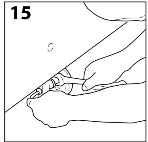
Using 17mm spanner and 6mm allen key, loosen nut on left side of the wheel to free the axle from the wheel support bar.
